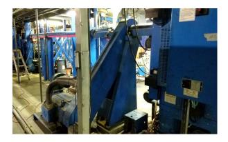
One (1) MasterFlo Refrigerated fountain solution circulator system, with 5-ton refrigeration unit.
