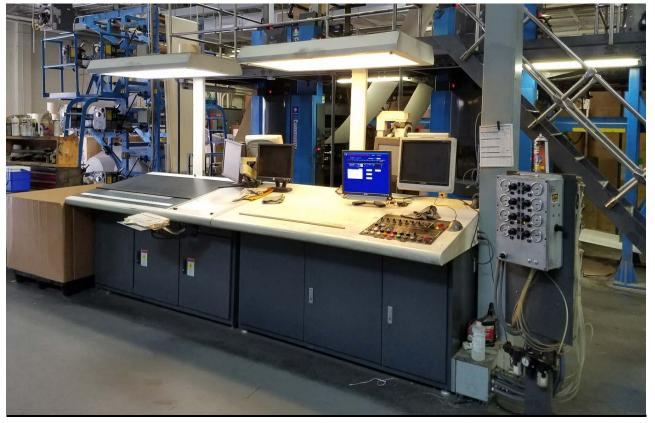
The press control system includes one (1) console to control the basic press functions and for quality control functions.
